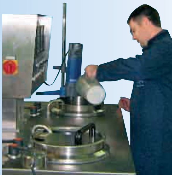
IKA® R&D bitumen emulsifying plant EPB 200 used in a pilot plant
